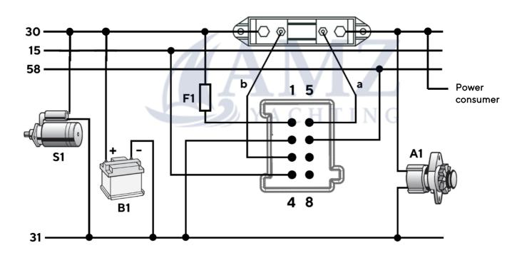
The starter current should not go through the shunt.
